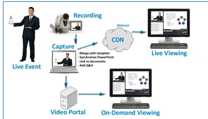
Figure 2 – the Webcasting production and archiving cycle
